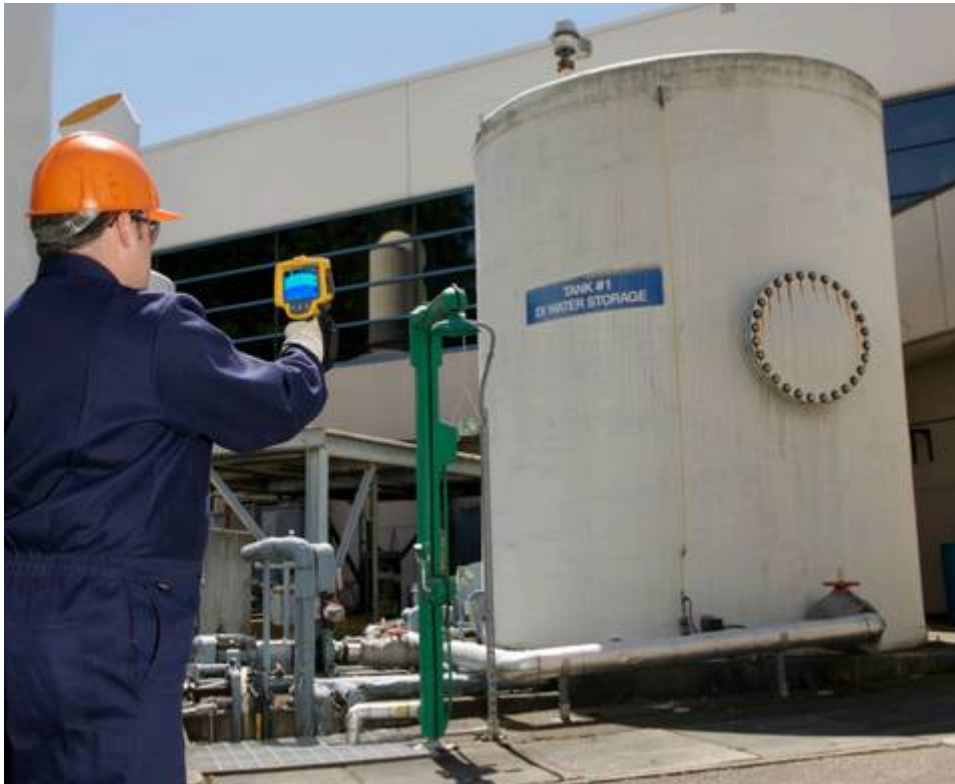
Thermal imagers can detect the level of fluid or other substance inside a tank, providing there is a temperature difference between the liquid, the air inside, and the air outside, and providing the tank is not made of a shiny material.
